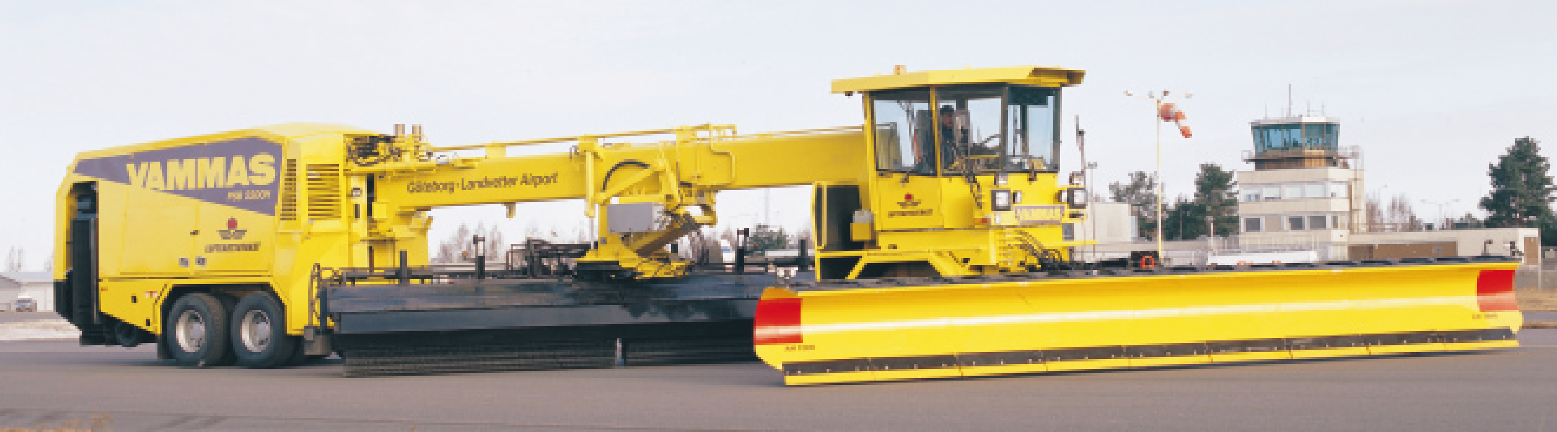
Finnish Vammas PSB 5500H, high-speed runway clearing unit for airports. Twin charge cooled Scania 14-litre V8 engines.
